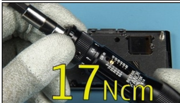
40. Check the torque of the tool.
